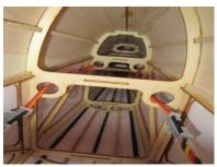
• insert the carbon fiber stabilizer tube into the pre drilled hole
