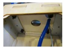
• Run the vent and fuel supply line to the bottom and side of the fuselage place a vent line end on the vent line and attach to the fuselage. Use a fuel dot on the fuel fill line. Ensure that on the fuel fill line that you install a Gas safe fuel filter inline.
