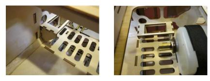
• Locate the Engine access hatch and use self-ta screws to tightly secure to the engine mount mount box.
