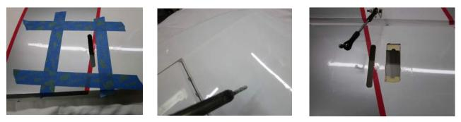
• prepare your servo buy centering it and adding your control horns along with a 6" Twisted Wire servo extension and a servo safety clip (sold separately at RedWing RC)
