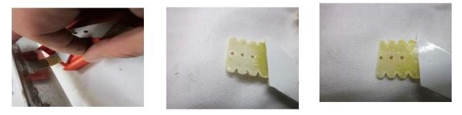
• Prepare the control horns and slots as you did in the wing installation. Once your comfortable with the way everything fits glue in the control horns, hinges and rudder to the fuselage
