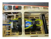
• Locate the carburetor supply nipple on the tank and run your line through the firewall to the carburetor
