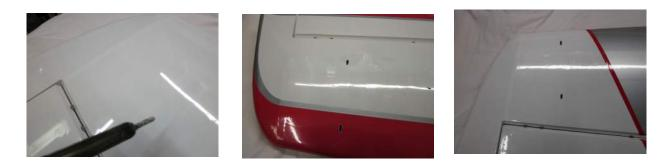
• Insert the pre painted metal SFG mounts through the holes you just made and run the bolts through the SFG and tighten into the mounts both top and bottom of wing.
